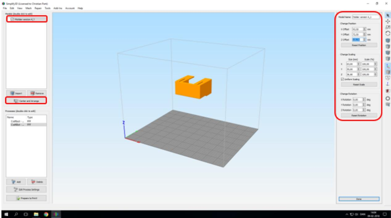
When part is oriented correctly (Make sure Z-offset is at 0), press “Prepare to Print!”
