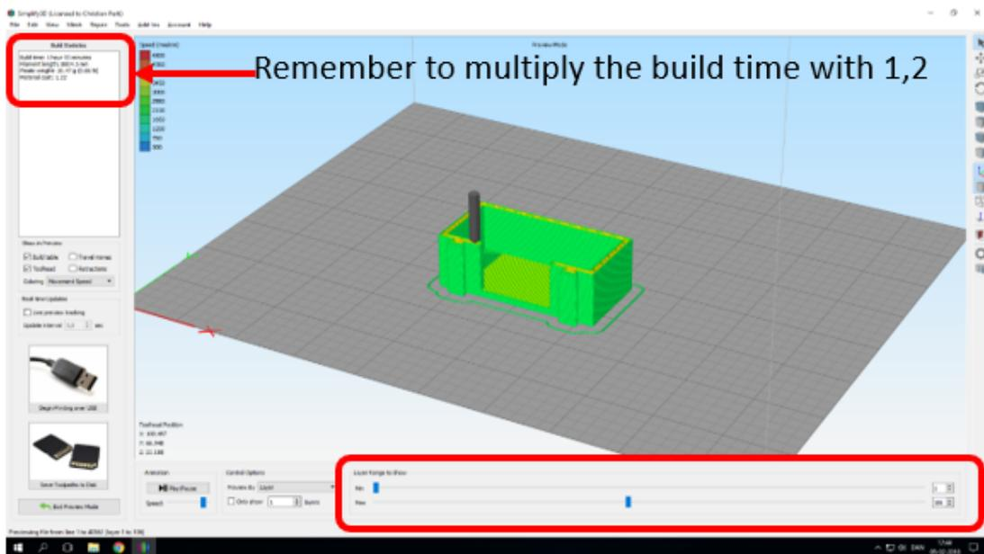
In the upper right left corner an estimated print-time, material usage and material cost are shown. These are only guidelines, which is why the time should be multiplied by 1,2 when determining time needed to print your part(s). Use the multiplied time-estimate for booking, adding the time necessary for slicing, starting the printer etc.
