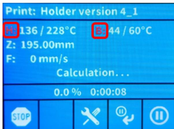
The display will now show an interface, where among other information the temperature of the bed and nozzle is shown. The temperature of the bed and nozzle will rise to the temperature shown to the right, and the print will start. Keep your fingers out of the printer while it's printing.
