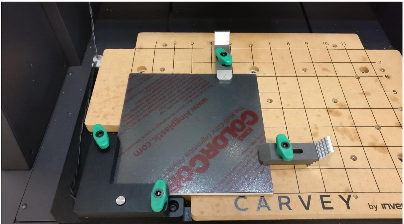
When the material is placed correctly, it is time to secure it doesn't move when the machine is running. For this we use the supplied clamparms, clampbases and clampbolts. Please choose sizing of these according to the size of your material.
