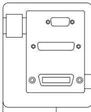
**TDS2CM Communications Extension Module.** The TDS2CM Communications module plugs directly into the rear panel of any TDS 200-Series oscilloscope. This module provides full GPIB and RS-232 compatibility and a Centronics port for hard copy output.
