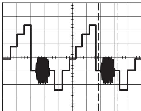
9. Push the **Window** button to see the expanded portion of the waveform.
