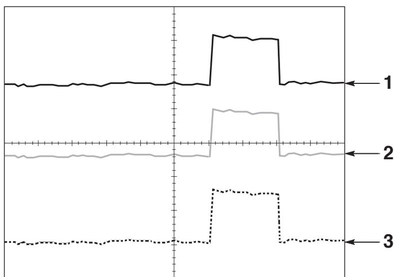
1. A solid black waveform indicates a live waveform display. The waveform remains black when the acquisition is stopped if no controls are changed that make the display accuracy uncertain.
