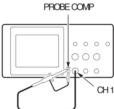
2. Set the switch to 10X on the P2100 probe and connect the probe to channel 1 on the oscilloscope. To do this, align the slot in the probe connector with the key on the CH 1 BNC, push to connect, and twist to the right to lock the probe in place.
