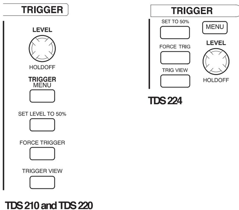
**LEVEL and HOLDOFF.** This control has a dual purpose. As an edge trigger level control, it sets the amplitude level the signal must cross to cause an acquisition. As a holdoff control, it sets the amount of time before another trigger event can be accepted. Refer to *Holdoff* on page 13 for more information.
