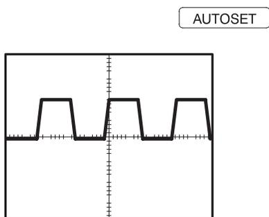
3. Push the **AUTOSET** button. Within a few seconds, you should see a square wave in the display (approximately 5 V at 1 kHz peak-to-peak).
