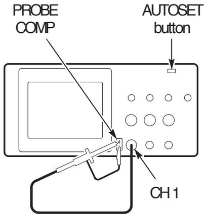
1. Set the Probe menu attenuation to 10X. Set the switch to 10X on the P2100 probe and connect the probe to channel 1 on the oscilloscope. If you use the probe hook-tip, ensure a proper connection by firmly inserting the tip onto the probe.
