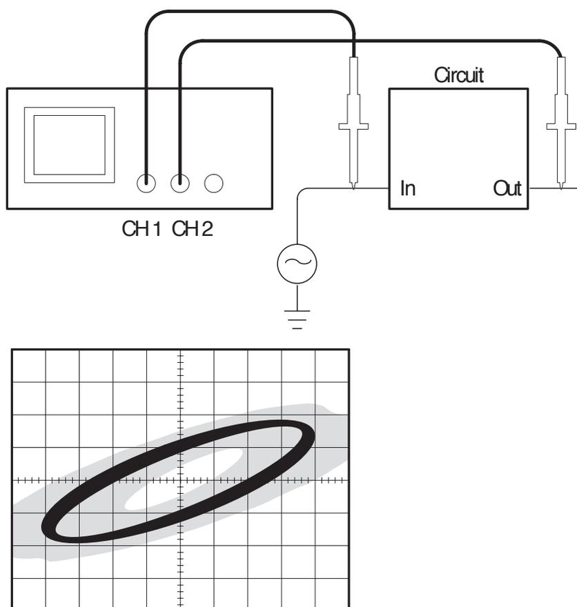
To view the input and output of the circuit in an x-y display, do these steps:
