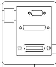
**TDS2MM Measurement Extension Module.** The TDS2MM module plugs directly into the rear panel of any TDS 200-Series oscilloscope. This module provides full GPIB and RS-232 compatibility and a Centronics port for hard copy output. The module allows measurement of rise time, fall time, and positive and negative pulse width. The module also provides Fast Fourier Transform (FFT).
