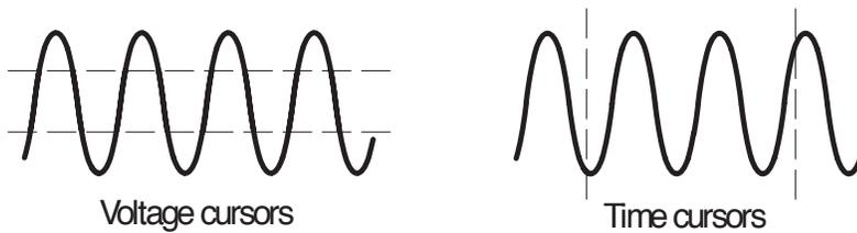
**U in Level and Delta Readouts.** Vertical sensitivity should match on waveforms used for math operations. If they do not match, and you use cursors to measure the waveform result of a math operation, an U displays that represents unknown.
