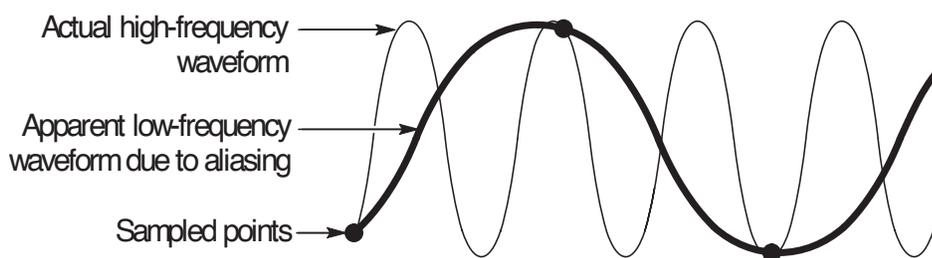
One way to check for aliasing is to slowly change the horizontal scale with the SEC/DIV knob. If the shape of the waveform changes drastically, you may have aliasing.
