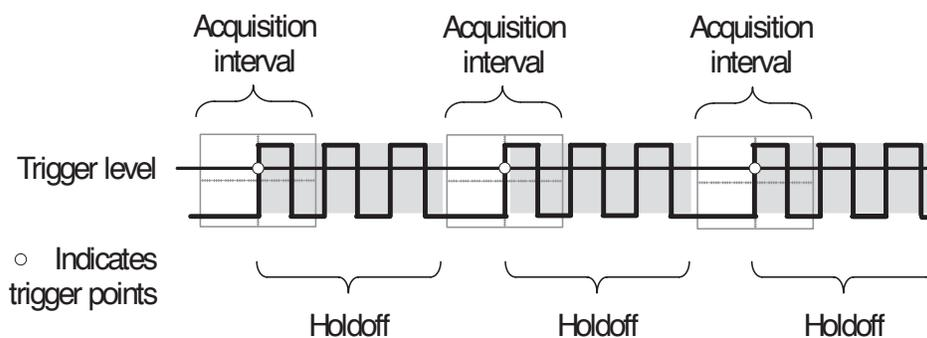
Triggers are not recognized during holdoff time.
