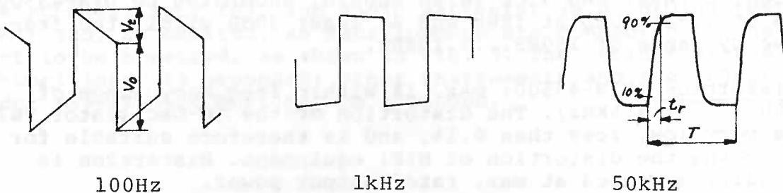
Fig. 5. Determination of  $f_l$  and  $f_u$
