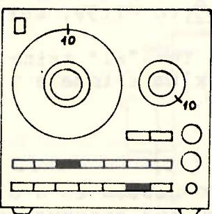
The co-axial output ⑦ is connected to a distortion meter capable of measuring distortion less than 0.03%. The pushbutton attenuator ⑫ is set on "1V". The variable attenuator ④ is set on "10". The frequency is adjusted to 1KHz. The potentiometer Pl is used to adjust to min. distortion. With the cabinet mounted it is checked if the distortion is still less than 0.03%.
