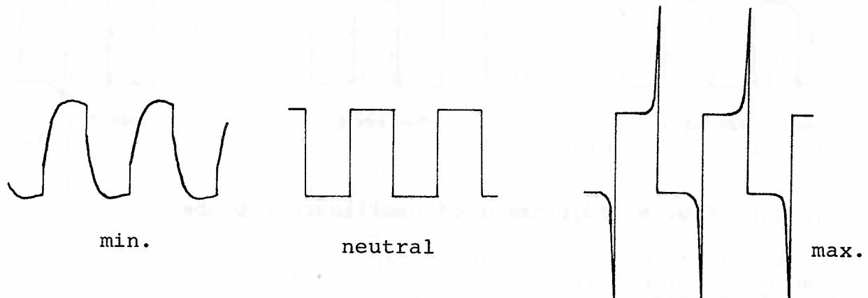
Fig. 7. Treble adjustment at  $f_L = 1\text{kHz}$
