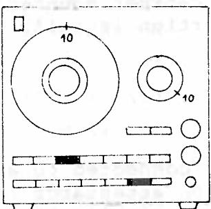
The co-axial output ⑦ is connected to a digital voltmeter. The pushbutton attenuator ⑫ is set on "1V". The variable attenuator ④ is set on "10". The frequency is adjusted to 1KHz (10Hz x 100).
