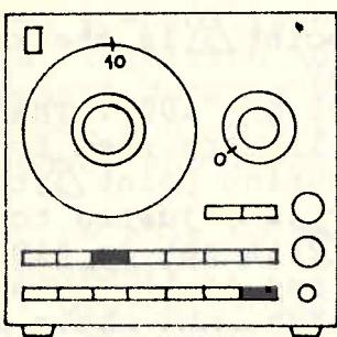
The pushbutton attenuator ⑫ is set on "3.16V". The variable attenuator ④ is set on "0". The frequency is adjusted to 1KHz. The potentiometer P4 is used to adjust the voltage across the resistor R68 to 50mV DC. The voltage is measured by a multimeter connected direct across the resistor.
