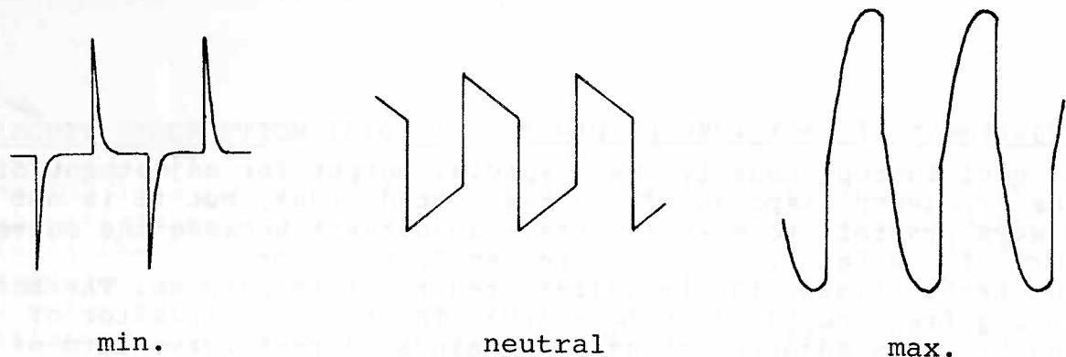
Fig. 6. Bass adjustment at  $f_L = 100\text{Hz}$
