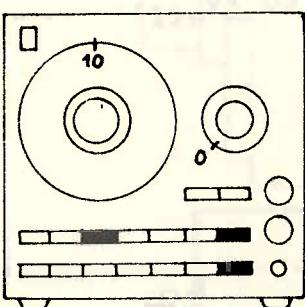
The co-axial output ⑦ is connected to a DC voltmeter. The pushbutton attenuator ⑫ is set on "3.16V". The variable attenuator ④ is set on "0". The frequency is adjusted to 1KHz. The  $\text{~v}/\text{v}_0$ -button is depressed. The potentiometer P7 is used to adjust the offset-voltage to 0V +/-50mV.
