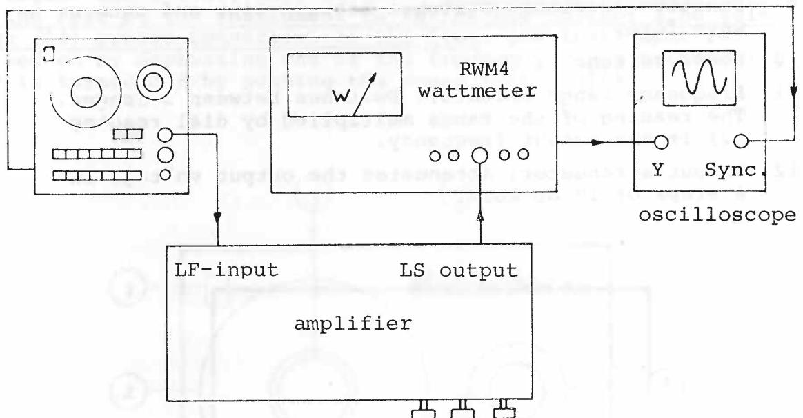
Fig. 3. Measuring set-up
